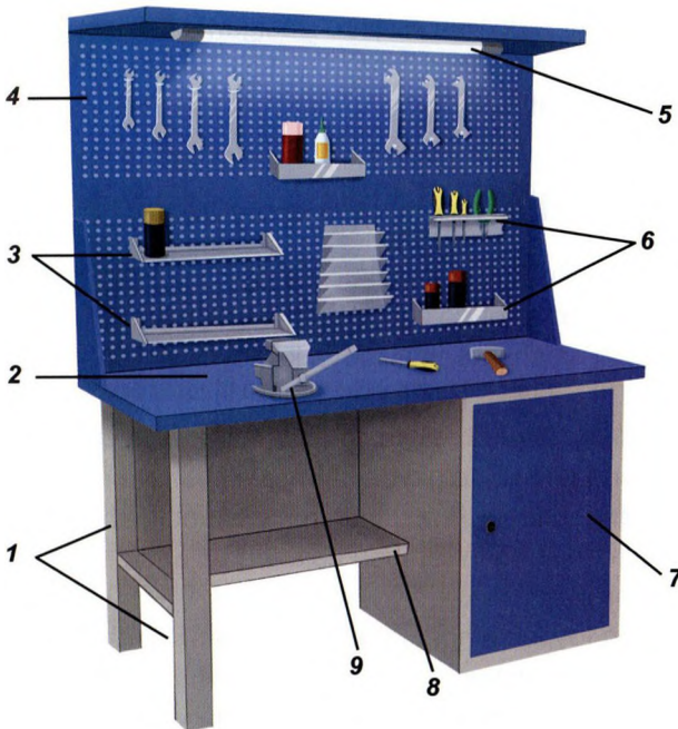
44-rasm. Chilangarlik dastgohining tuzilishi:
